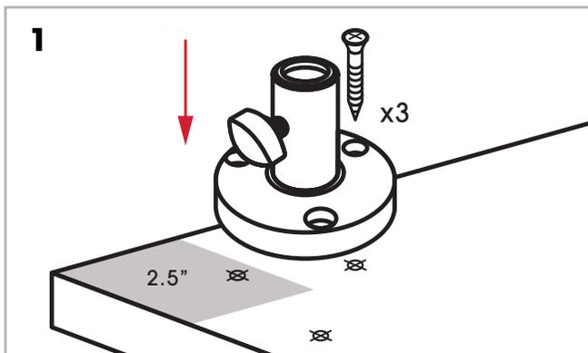
Place surface mount at least 2.5" from the edges of the desk. Then, use a screw driver to secure the surface mount.
