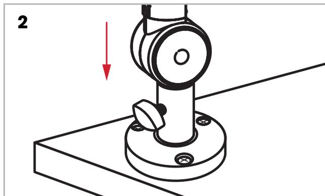
Insert the arm into the hole in the top of the surface mount desk insert.
